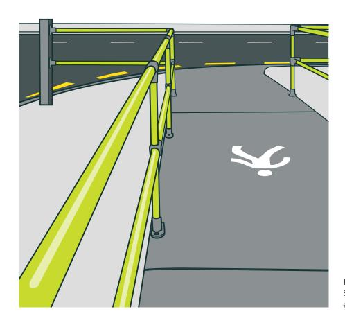
**FIGURE 7:**Separate work site entry for pedestrians
