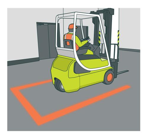
FIGURE 17: Forklift with projected laser light
